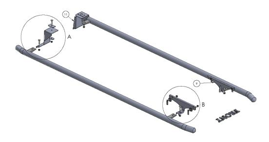
After mounting sidebars, make sure sidebars and brackets are in right position with the body of your van
