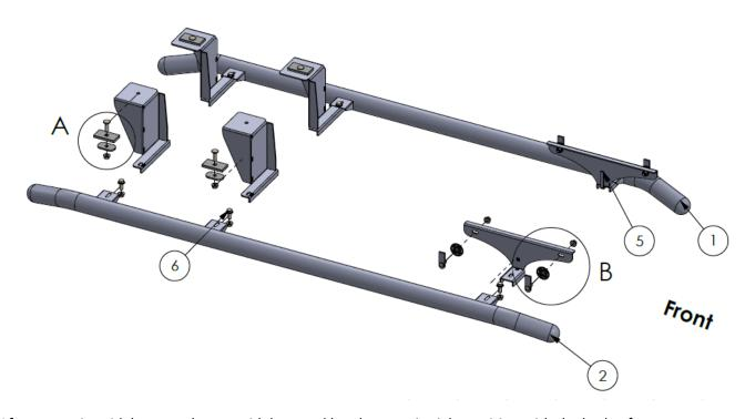
After mounting sidebars, make sure sidebars and brackets are in right position with the body of your van
