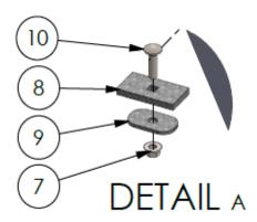
Place rearbracket, ad mounting plate 9 and hand tighten with M10 nut
