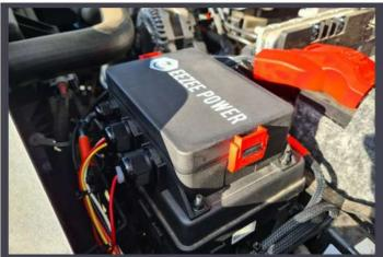
Find a good place to mount the relay box and mark the mounting holes. Tip: cover the area with painter's tape before making the marks. Drill the holes with a 5mm drill bit.
