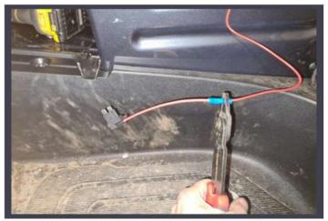
Place the car's fuse in the bottom place of the Add-a-fuse tool. Crimp the Add-a-Fuse tool onto the ignition cable (cable number 4 - see diagram on page 3).
