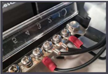
Loosen the screws a few turns, slide the cable connector underneath and tighten the screws.
