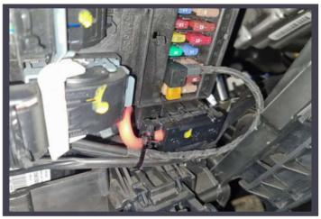
Place the Add-a-Fuse tool in the original position of the car's fuse.
