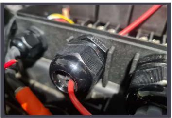
Remove the rubber plugs and place the positive cable of the 12V accessory through the provided holes. Attention: never connect accessories with more than 30A!
