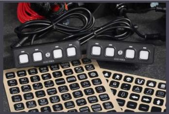
Now install the sticker on the button that corresponds to the 12V accessory. Never remove a sticker with a sharp object (such as a knife) as this can damage the switch panel!
